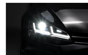
LED Position Light and Xenon Low Beam
