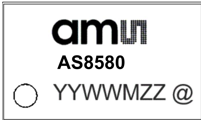
Figure 27: Marking of plastic production parts (top view)
