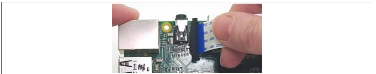
Figure 5: Insertion of camera cable
