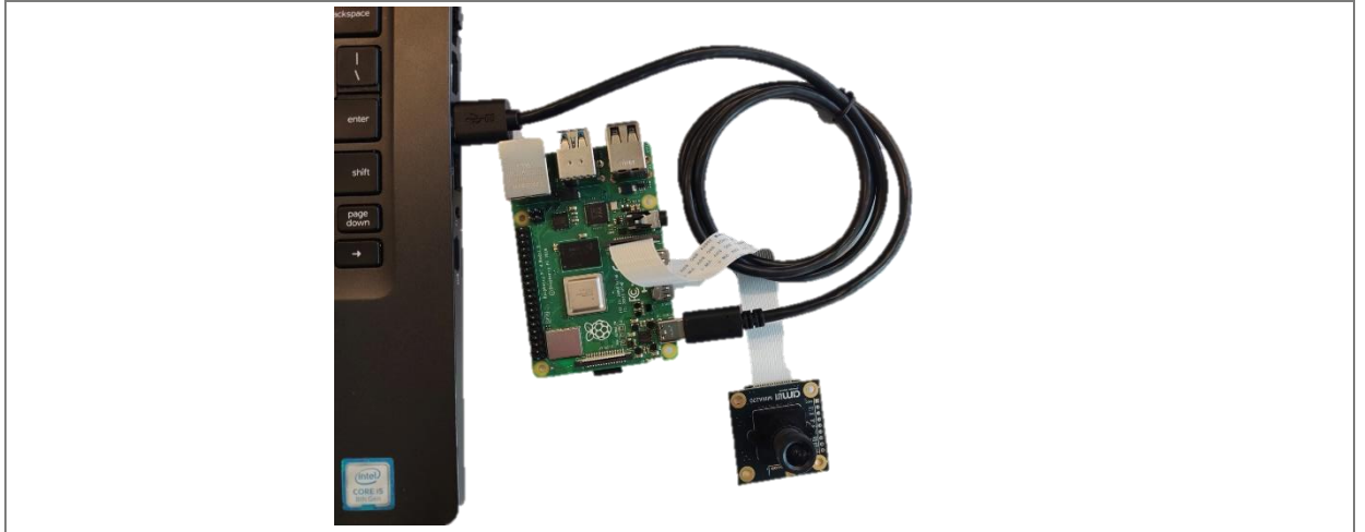
Figure 3: Connection of hardware components
