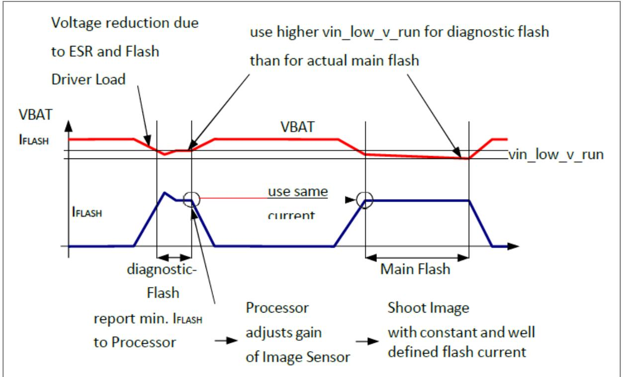
The different settings for  $vin\_low\_v\_run$  allow a constant main flash current without dropping  $V_{IN}$  below  $vin\_low\_v\_run$ .
