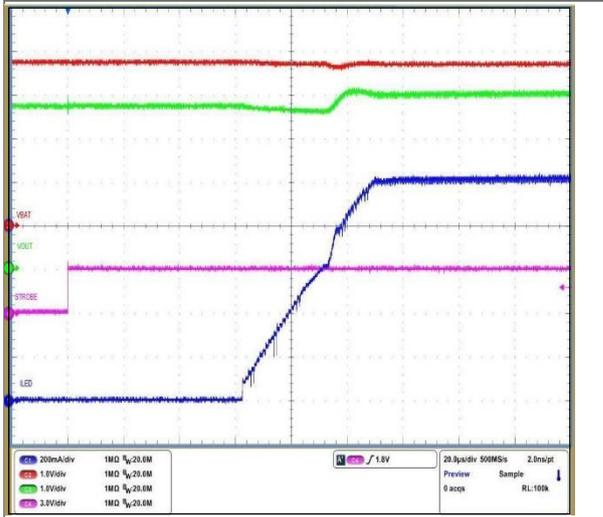
Figure 9: I<sub>VIN</sub>, I<sub>LED</sub> STARTUP (I<sub>LED\_OUT</sub> = 800 mA)
