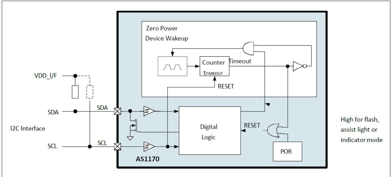
In shutdown mode once pin SCL goes high for the first time, the internal counter shown in Figure 20 is immediately reset thus releasing the internal RESET (assuming  $V_{IN}$  is above  $V_{UVLO}$ ) signal and allows instant communication on the I<sup>2</sup>C bus. Therefore, no additional action is required to leave the shutdown mode and start I<sup>2</sup>C communication.
