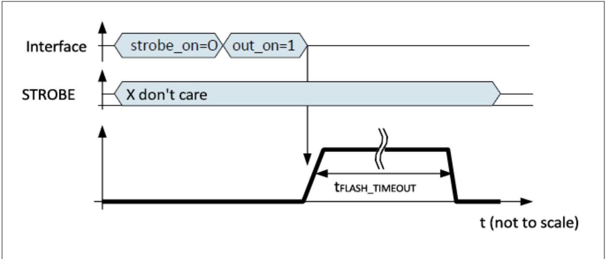
Figure 25: AS1170 flash duration defined by flash\_timeout, starting with STROBE rising edge
