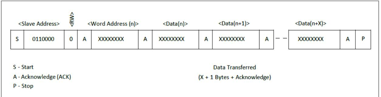
Figure 30: Data read (from current pointer location) - slave transmitter mode
