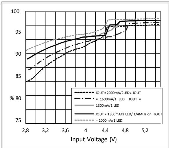
Figure 5: Application efficiency ( $P_{LED}/P_{VIN}$ ) vs.  $V_{VIN}$
