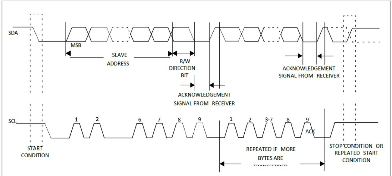
Depending upon the state of the R/W bit, two types of data transfer are possible:
