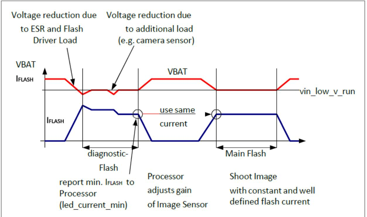
If the diagnostic flash should be short (e.g. 10 ms) it is recommended to operate this diagnostic flash at slightly higher vin\_low\_v\_run setting compared to the main flash.
