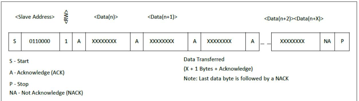
Figure 31: Data read (write pointer, then read) - slave receive and transmit
