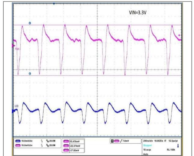
Figure 12: I<sub>LED</sub> rampdown (ILED\_OUT = 1.0 A)
