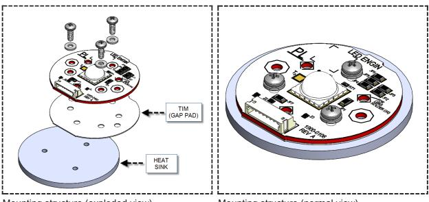
Mounting structure (exploded view)
