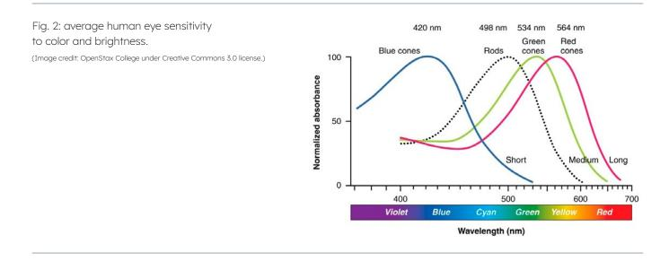
The human brain can fuse the inputs from the eye's blue, green and red cones to produce a color sense output, but it cannot distinguish the complex pattern of color peaks and troughs which distinguish a white LED from a fluorescent lamp, when both have average peak output at around 540-580nm, perceived as a blue-green white.
