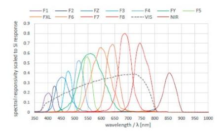
Fig. 5: the spectral sensitivity of the AS7343 multi-channel spectral sensor
