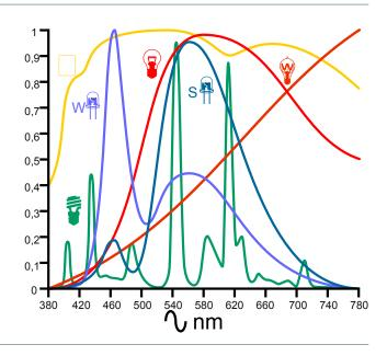
What is striking about the graph is that each light source's curve has a distinctive shape, and concentrates its radiant power in different parts of the spectrum. This explains why each source has different perceived color effects.
