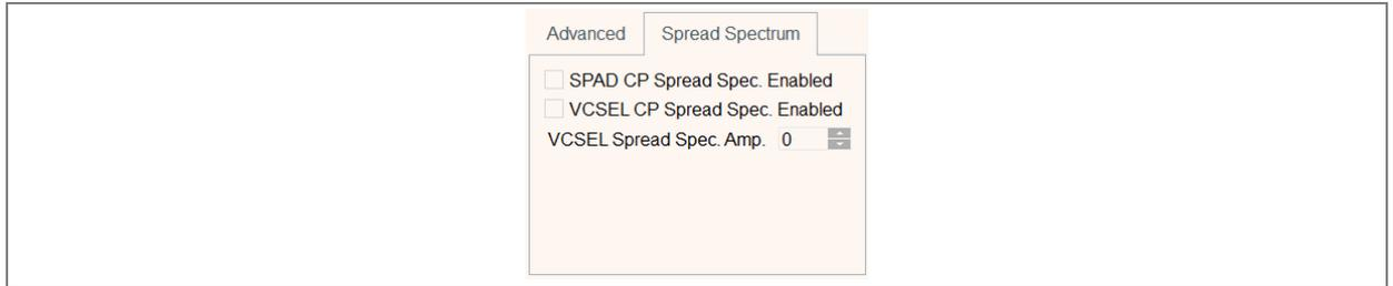
These controls enhance the EMC performance of the sensor. There's one control for each hardware block. The GUI selects the recommended configuration for these blocks. Please refer to the datasheet for more details.
