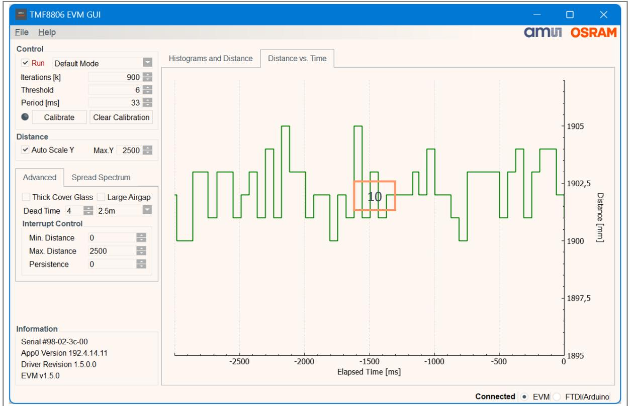
The “Distance vs. Time graph” (10) replaces the “Distance graph with confidence” and histogram graph with a single display of the object data reported over the previous three seconds.
