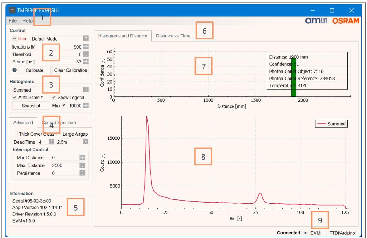
The “Histogram graph” (8) shows time-to-distance-converter (TDC) histogram information. The X-axis indicates the “time buckets” in multiples of 100 picosecond increments (200ps in 2.5m mode, 400ps in 5m mode, 800ps in 10m mode). The Y-axis indicates the number of photonic triggers / hits at the given time interval.
