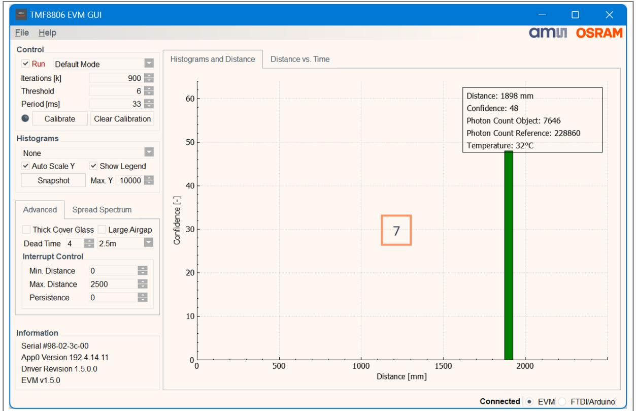
The “Distance graph with confidence” (7) is a plot of the detected object’s distance vs. the confidence value (range 0 – 63) of the given detection. The X-axis indicates the distance in millimeters and the Y-axis indicates the confidence value.
