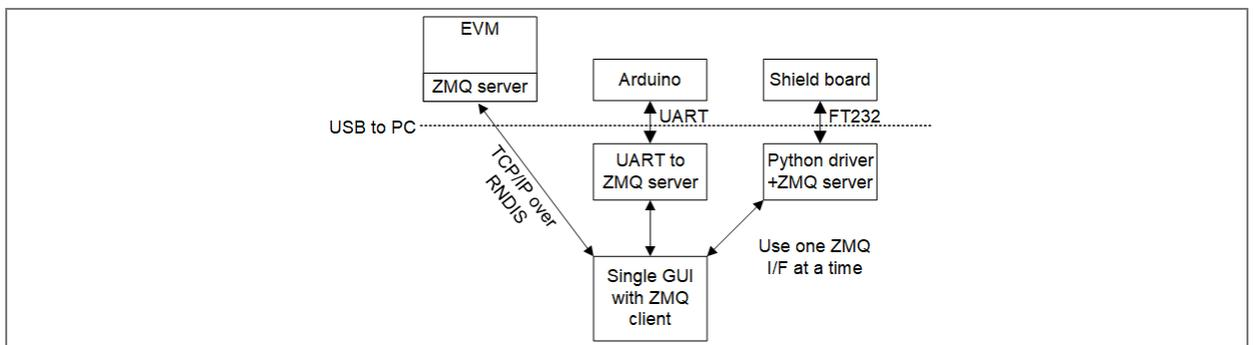
The abbreviation ZMQ in Figure 2 stands for ZeroMQ. ZeroMQ is used as central communication technology for the EVM software stack.
