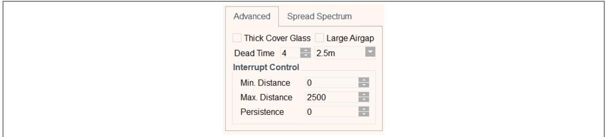
There are two tabs with controls in this part of the GUI. One tab with advanced settings that influence the sensor measurement and one tab with controls for EMC performance enhancements.
