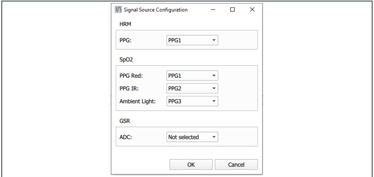
“SpO2” is for configuring the SpO2 Parameters. Enter the parameters associated with the specific settings of the AS7050 in the SpO2 configuration settings. Due to production and assembly tolerances, it is recommended that the below-mentioned factors for the photodiode offset current compensation ( $PD_{off\_fact\_red}$  and  $PD_{off\_fact\_ir}$ ) are determined for the device under development; after the sensor has been integrated and the optical configuration is finalized.
