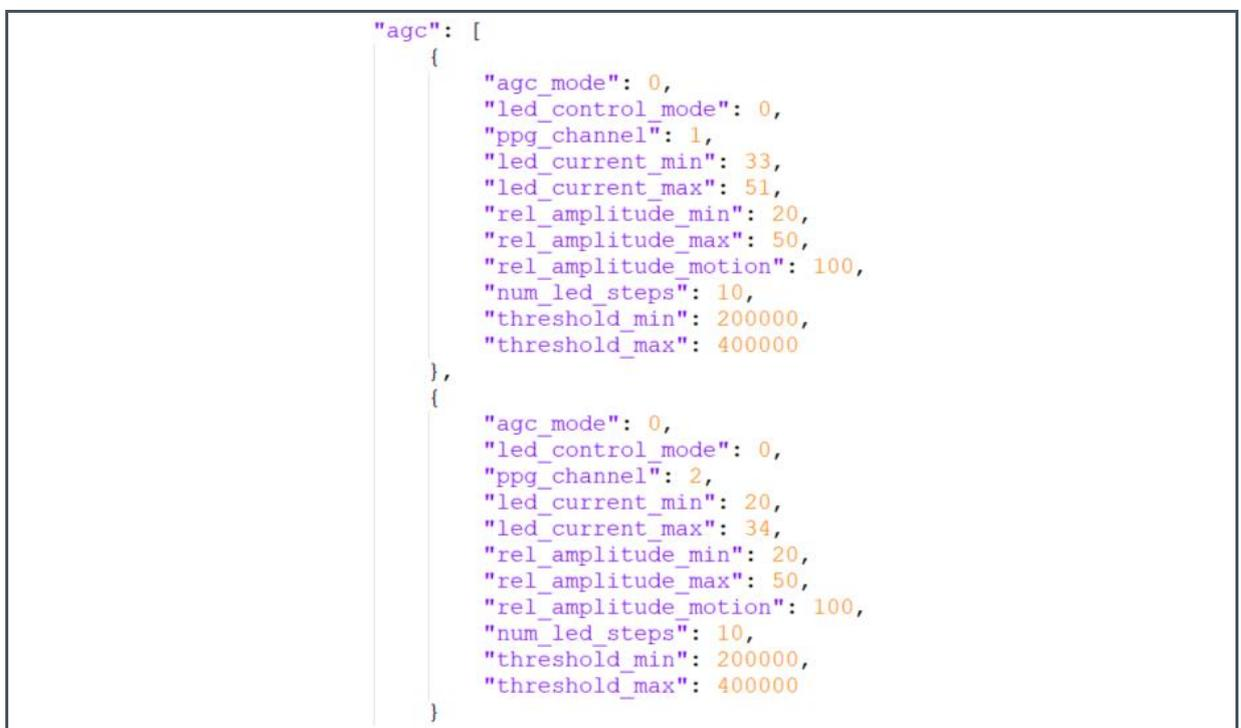
The PD offset and LED current control is an algorithmic approach to increase the signal quality of the PPG signals. The algorithm continuously monitors the ADC outputs and, if necessary, reconfigures the AS7050 while measuring to ensure ideal conditions.
