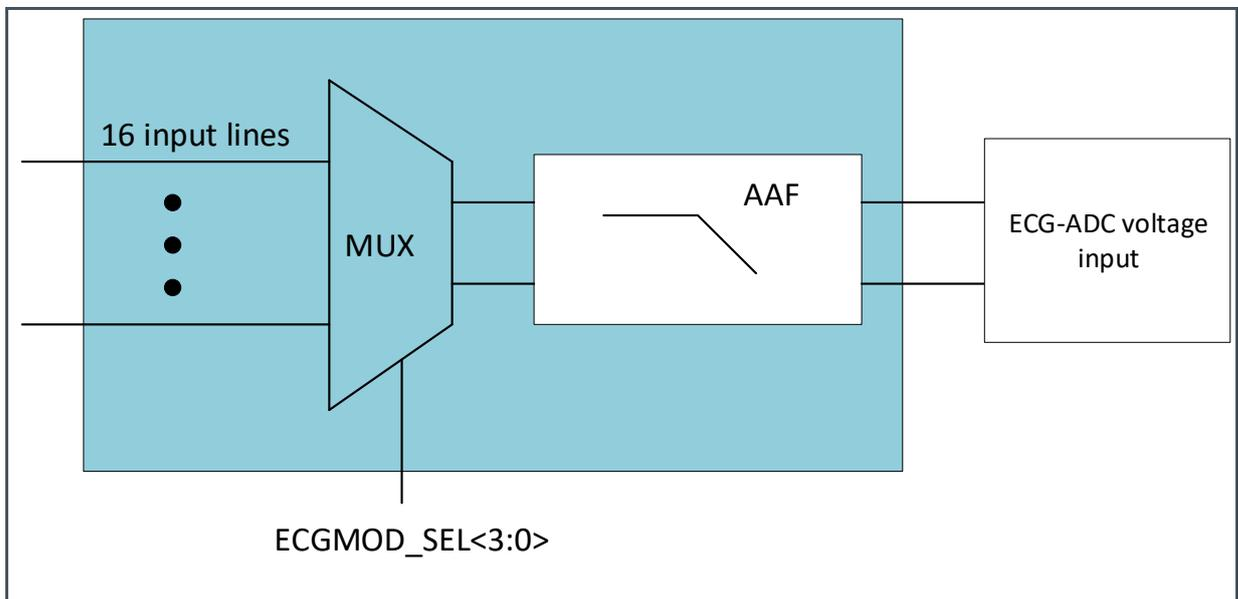
ECG modulation can be enabled to modulate the ECG signal. DSM gain can also be enabled. An anti-aliasing filter (AAF) is used in the ECG-ADC input selection before the signal sampler or ECG-ADC voltage input to restrict the bandwidth of a signal and satisfy the band over the band of interest.
