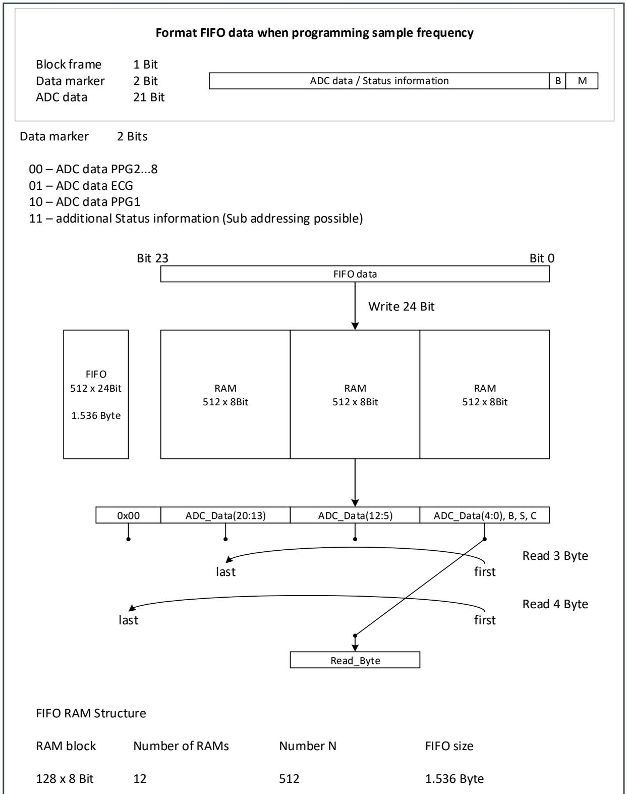
The AS7050 FIFO is 1536 bytes long. ADC samples are 3/4 bytes, which means the FIFO can hold up to 512 samples. There is a FIFO length register, which indicates how many samples are currently available in the FIFO. The FIFO can send an interrupt when the number of available samples reaches a certain configurable threshold.
