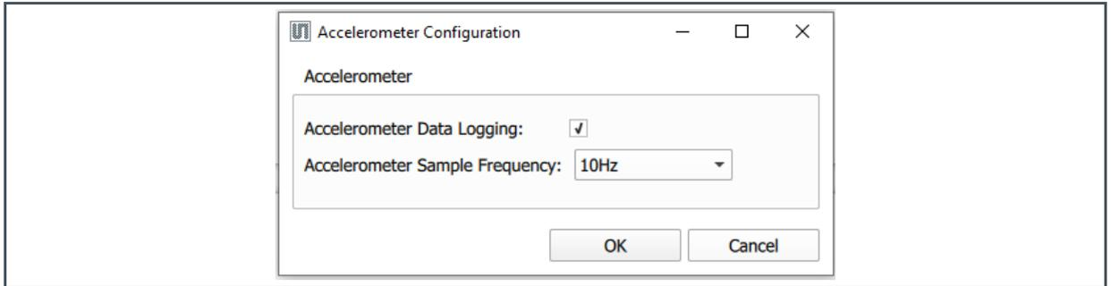
The accelerometer is used for displacement information. The HRM application includes this accelerometer data and makes the accelerometer useful and practical.
