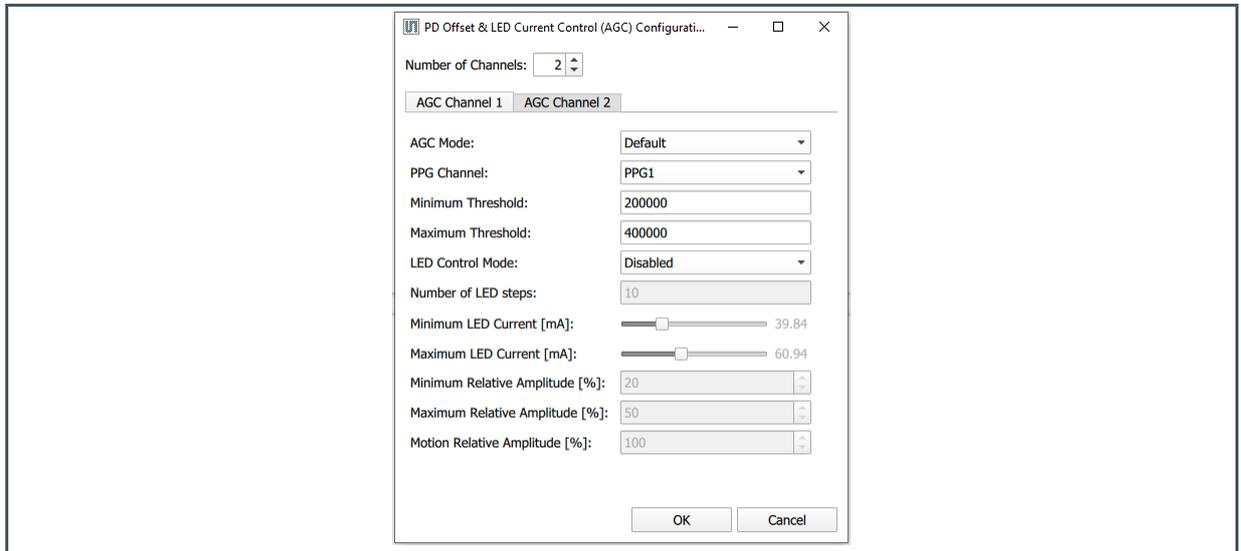
The firmware supports up to four AGC instances, each running independently. Thus each AGC instance controls a single PPG channel, up to eight different PPG channels can be controlled by the AGC.
