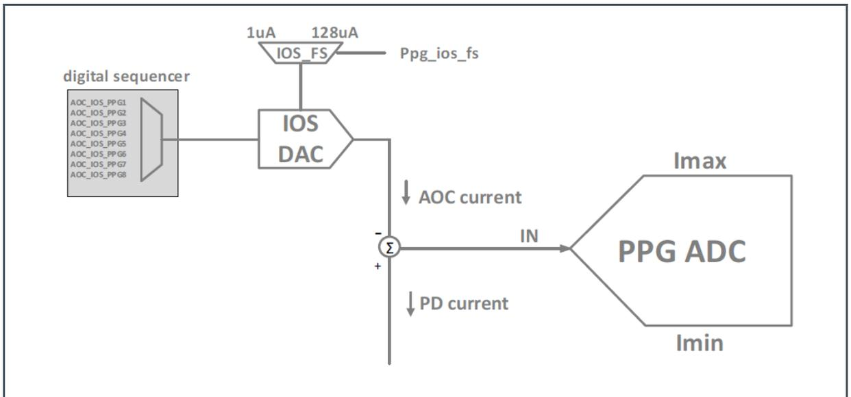
Ambient light can be compensated for each subsequence, either directly by writing a value from 0...255 to AOC\_IOS\_PPGi digital register values, or by a digital regulation loop.
