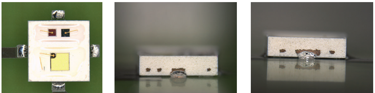
Figure 9: Solder side wetting structure for solder joint inspection
