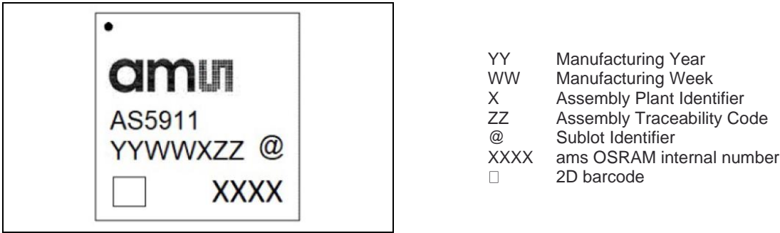
Figure 3: FBGA400 package marking/code of AS5911
