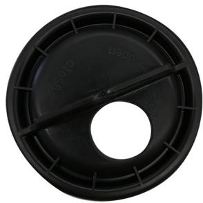
Mark the headlight protective cover where the hole needs to be drilled (13 mm from the center toward the right). Using a step drill, drill the hole needed for the cable to pass through.<sup>3)</sup>
