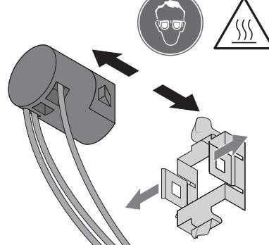
Disconnect the halogen adapter from the plug.<sup>5)</sup>
