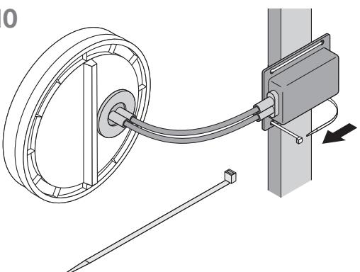
**Mount the SMART CANBUS (load resistor) to the vehicle's body (metal).**
