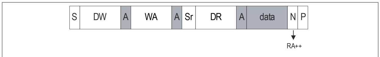
Figure 55: I 2 C random read format
