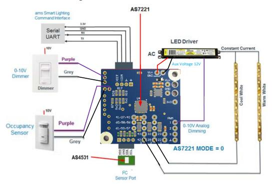
As shown above, a Color Tuning AS7221 SLIK adds Daylighting with a simple inclusion of an AS4531 via I<sup>2</sup>C:
