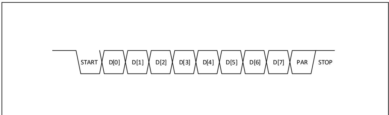
The PAR bit is even parity calculated over the data bits (D[0:7]). Each frame is transferred from LSB to MSB.
