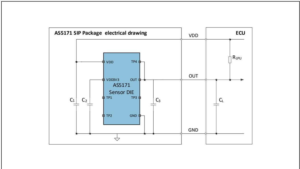
Figure 43 and Figure 44 show the recommended schematic in the application. C<sub>1</sub>, C<sub>2</sub> and C<sub>3</sub> are Built-in capacitors in the SIP Package as shown in Figure 49.
