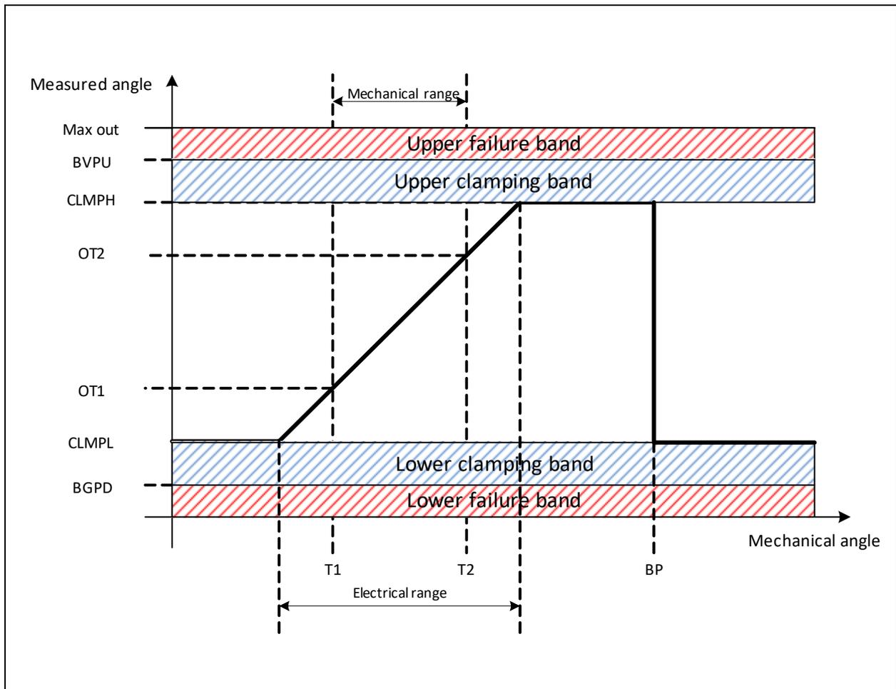
The breakpoint **BP** sets the discontinuity point where the output jumps from one clamping level to the other. It is strongly recommended to set the breakpoint at the maximum distance from the start and stop position (**T1** and **T2**). To handle the case of a full turn, a hysteresis function across the breakpoint can be used to avoid sudden jumps between the lower and upper clamping level.
