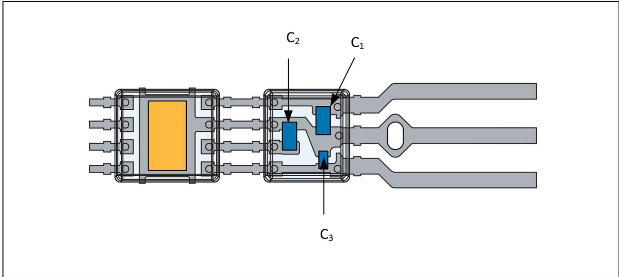
The built-in capacitors are ceramic multilayer type X8R. The capacitors build for high temperature applications up to 150°C
