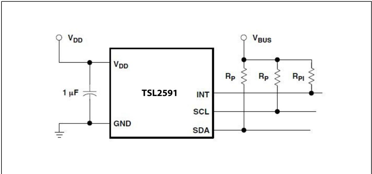
The I<sup>2</sup>C signals and the Interrupt are open-drain outputs and require pull-up resistors. The pull-up resistor ( $R_p$ ) value is a function of the I<sup>2</sup>C bus speed, the I<sup>2</sup>C bus voltage, and the capacitive load. The ams OSRAM EVM running at 400 kbps, uses 1.5-k $\Omega$  resistors. A 10-k $\Omega$  pull-up resistor ( $R_{pI}$ ) can be used for the interrupt line.
